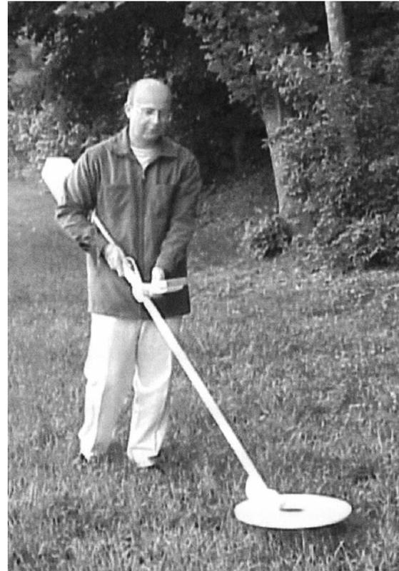
Fig. 1. GEM-3 monostatic broadband EMI sensor.
