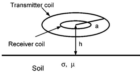
Figure 1. A concentric coil sensor over a half-space.
