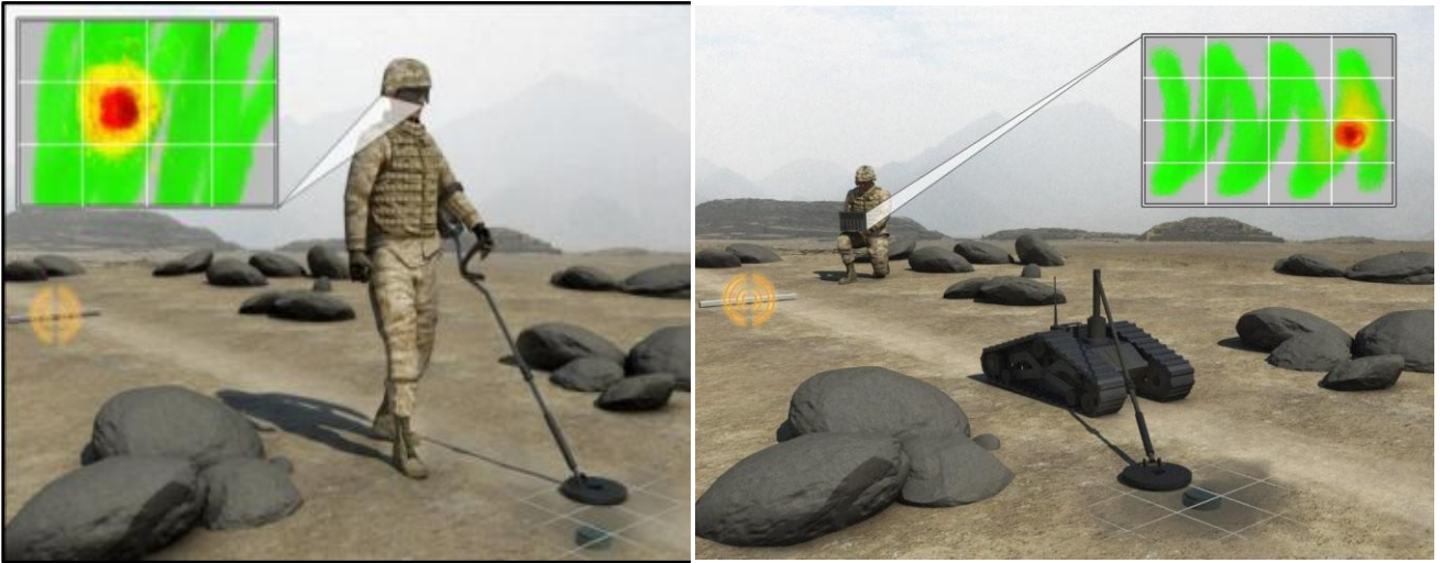
Fig 5. The GEM-3M displays visual ground image following the sweep paths
