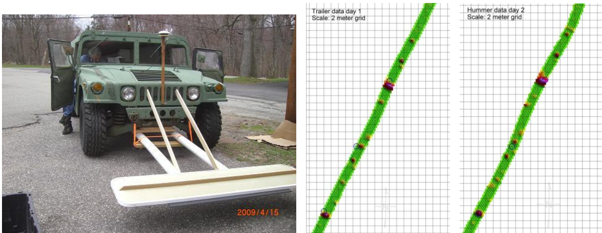
Fig 1. A prototype GEM-3 array mounted on a Hummer for a demo in Picatinny Arsenal. Shown on the right are realtime GPS-based ground image over a seeded roadway traversed on two different days. Notice the excellent data repeatability.
