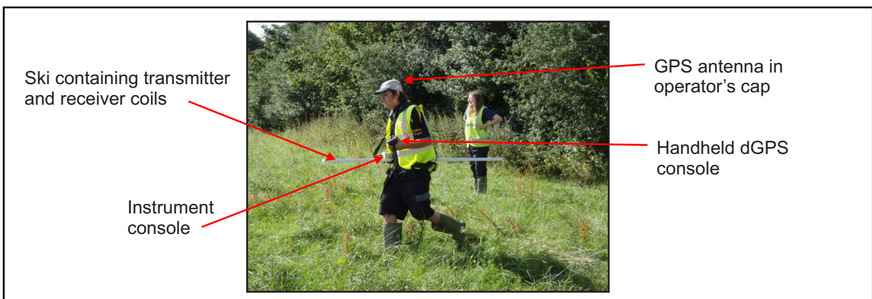
Figure 1: A GEM-2 survey in progress using a vertical dipole/horizontal coil orientation.
