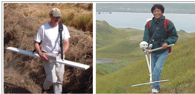
Figure 1. Portable, digital, broadband EMI sensors. The instrument in the left photo has three linearly spaced coils with a maximum separation of 1.67 m. The concentric instrument in the right photo comes in three disk sizes up to 96 cm in diameter. The largest one is typically cart-mounted.
