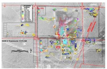
Because of its sensitivity, programmability, and ease of use by a single person in difficult terrain, the GEM-2 can greatly reduce the cost of many surveys. The complete paper can be found in the FastTIMES archive at <a href="https://enengs.memberclicks.net/latest-issue">https://enengs.memberclicks.net/latest-issue</a>. The survey was carried out by Icon Environmental Services ( www. Iconenv.com ).
