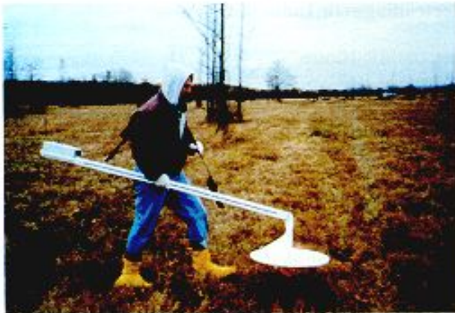
Figure 1. GEM-3 in operation. The entire unit weighs about 9 lbs and has a data-logging capacity of about 50,000 points before downloading.
