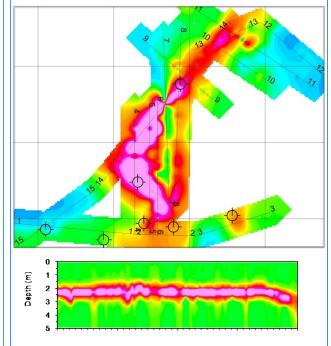
A conductivity-depth section defines the brine concentration at depths of 2–3 m, which was later confirmed by drilling.
