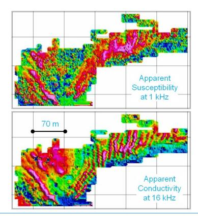
**Brine Contamination at an Oil Field:** The U. S. Geological Survey (USGS) conducted a GEM-2 survey to characterize shallow brine contamination at an oil field in Oklahoma. Data were collected at five frequencies from 330 Hz to 47,010 Hz. The figures below show the apparent conductivity map at 14 kHz, which define the brine concentration in 3D.
