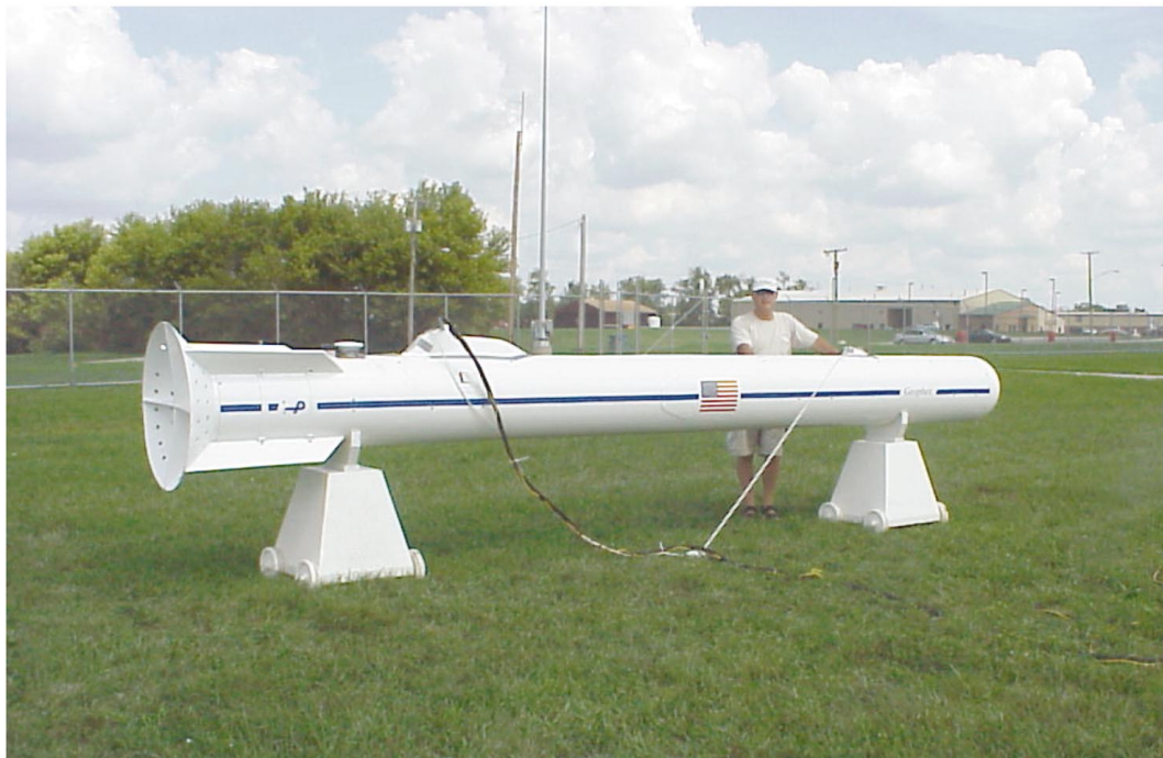
FIG. 1. GEM-2A sensor on the ground (bottom) and towed by a Bell Jet Ranger (top).
