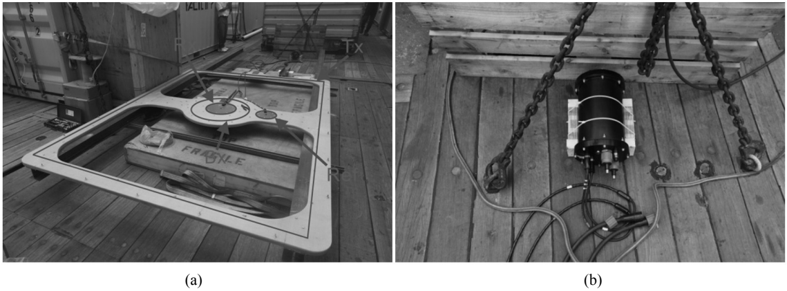
Fig. 2. (a) Assembled marine small loop electromagnetic survey equipment (KIGAM-GEM3). The Rx, Tx, Bx and Ref are receiver, transmitter, bucking and reference coils. (b) Pressure housing of control unit in the KIGAM-GEM3 system.
