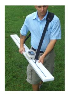
Because it is comfortable to carry and has a field-swappable battery, extended surveys are no problem. Its powerful transmitter and wide coil separation allow scanning to depths up to 10 meters, depending on soil conditions.
