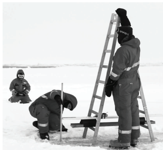
Fig. 2. Multi-frequency EM induction sounding data are recorded with the GEM-2 at different heights above sea ice. The signal directly depends on the distances to the conductive layers. Photograph by Sandra Schwegmann, 24 June 2013.
