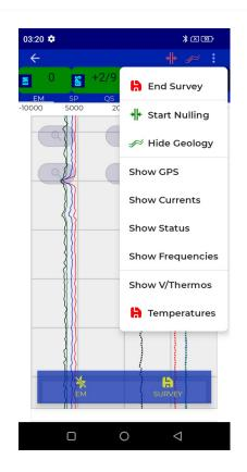
**The menu** can be opened by pressing the three dots in the top right and contains multiple commands, mostly useful for managing surveys. "End Survey" is used for closing the file after completing a survey.
